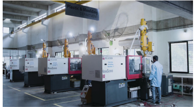
Plastic Enclosure Manufacturing In-house Injection Moulding
